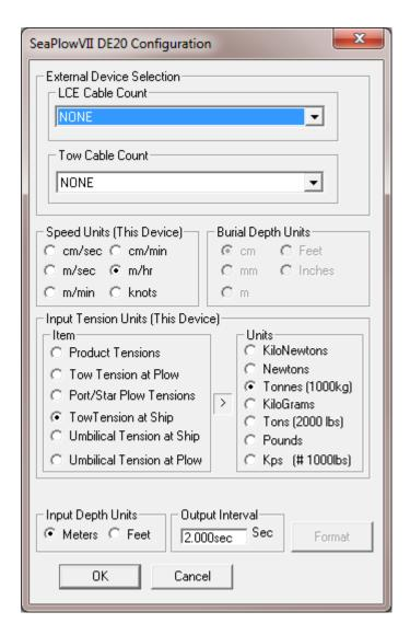
Select the data source for the LCE telephone cable count data and the Tow cable count data from the dropdown lists. Also, select the appropriate Input Speed Units, as well as the Input Tension Items and their associated Units. Specify whether the Input Depth Units are to be meters or feet.
