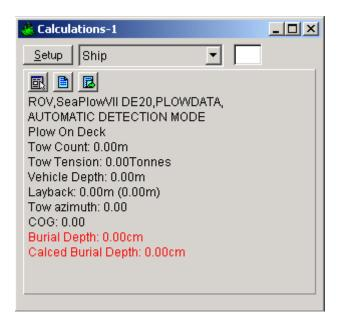
From this window, you can monitor some of the input data as well as the layback calculation. This Calculation window also provides a shortcut to the Configure Plow dialog box by clicking the button.
